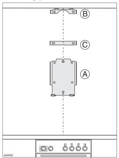
The ventilation system will be mounted to the wall through the use of retaining plates. Plate A is installed first, followed by plate B. Plate C should only be used if the distance between plate A and plate B is greater than 14  $^{3}/_{8}$ " (365 mm).
